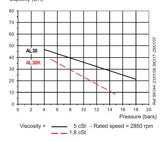
Data shown take into account a wear margin. Do not oversize the pump when selecting the gear capacity.
