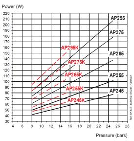
Viscosity = 5 cSt - Rated speed = 2850 rpm 1.8 cSt
