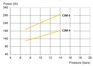
Viscosity = 0,75 cSt - Rated speed = 2850 rpm
