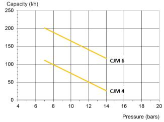
Viscosity= 0,75 cSt - Rated speed = 2850 rpm
