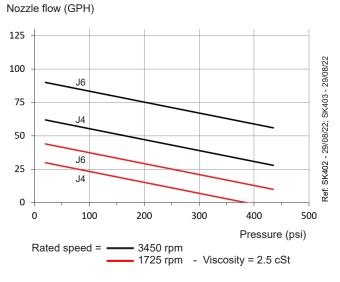
Data shown take into account a wear margin. Do not oversize the pump when selecting the gear capacity
