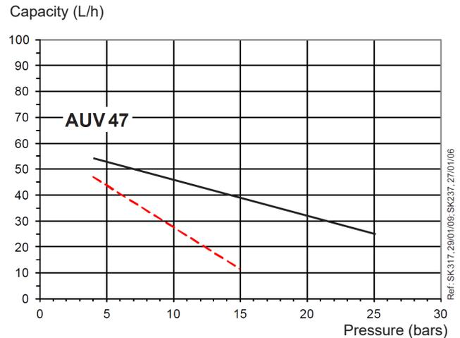
Viscosity = --- 1,8 cSt    Rated speed = 2850 rpm
