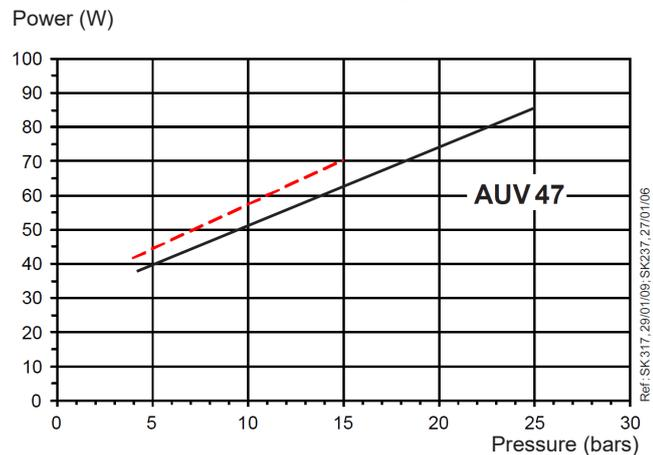
Viscosity = --- 1,8 cSt    Rated speed = 2850 rpm
