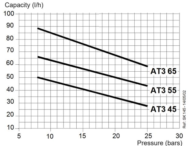
Viscosity = 5 cSt - Rated speed = 2850 rpm
