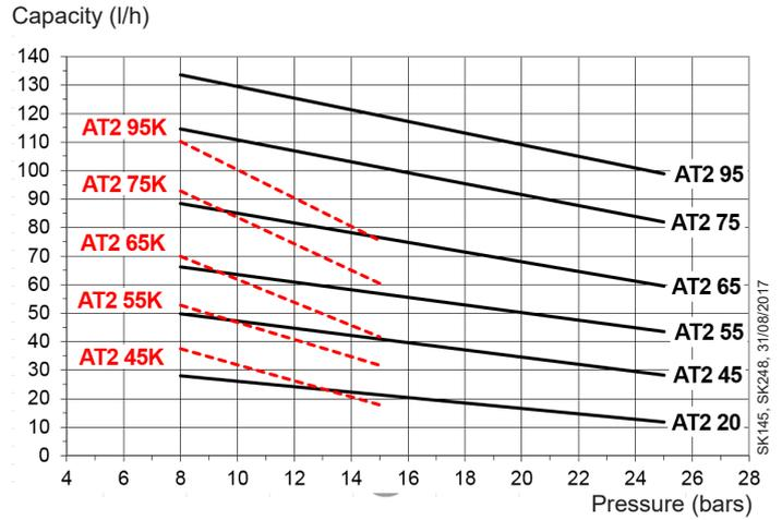
Data shown take into account a wear margin. Do not oversize the pump when selecting the gear capacity to ensure the optimum operation of the (NO) solenoid valve (switching low/high mode).
