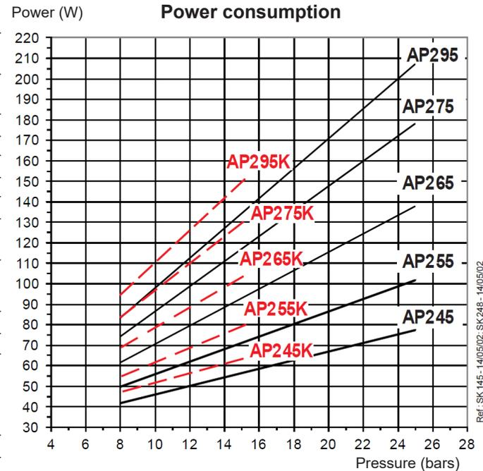
Viscosity = — 5 cSt - Rated speed = 2850 rpm
