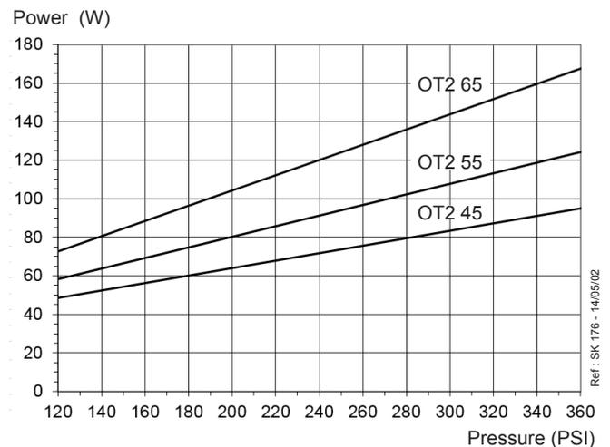
Viscosity = 5 cSt - Rated speed = 3450 rpm
