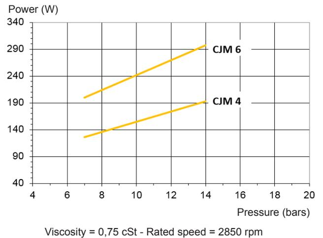
\* Data given for a Methanol blend with 91% Methanol, 3% Acetone, 3% Xylene, 3% Acetate. This blend may not be representative of the Methanol blend used in your market. Tests with local blend have to be performed before using the pump in a burner.
