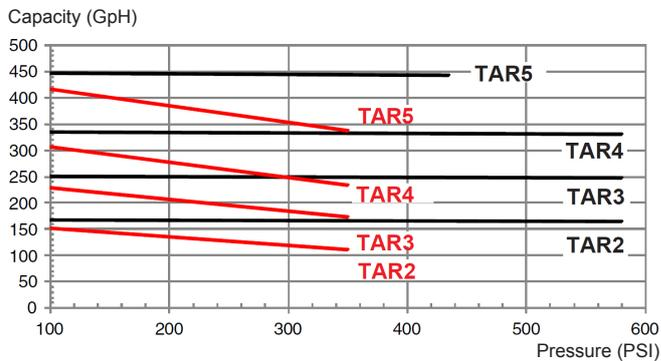
Data shown are for new pumps, with no allowance for wear.
