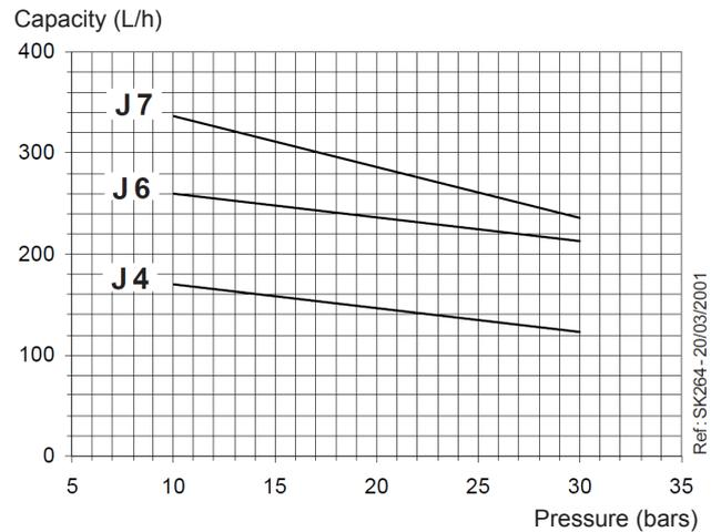
Viscosity = 5 cSt - rated speed = 2850 rpm
