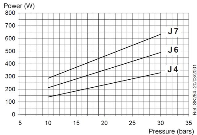
Viscosity = 5 cSt - Rated speed = 2850 rpm
